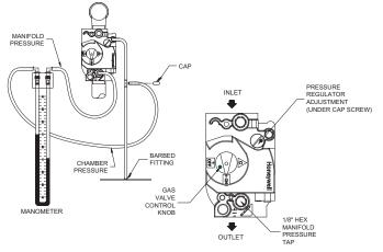
Figure 31 – Measuring Net Manifold Gas Pressure
